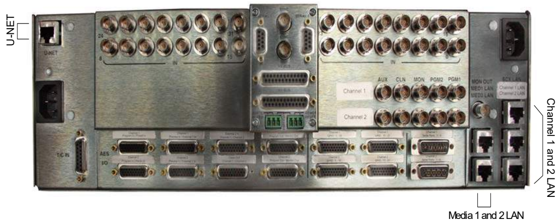
Figure 1-1. MC-4000 rear - UNET and Input connections
